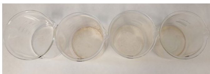
Figure 1. Global migration assay after dryness evaporation. From left to right: blank and three samples results after assay with granite test samples (samples 1, 2 y 3).
